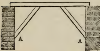
Fig. 100—Represents a horizontal beam C supported near the middle by inclined struts A, A.
